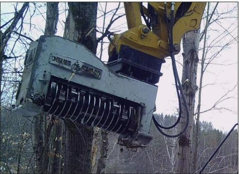
"Brontosaurus" mulching head/forestry mower is used to mechanically remove woody invasives
